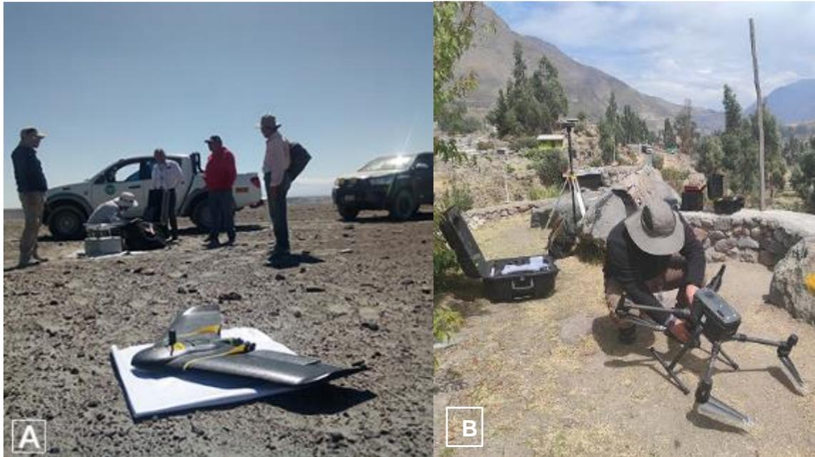
**Figura 6.** (A) Dron eBee Plus. (B) Drone Matrice 300 RTK
