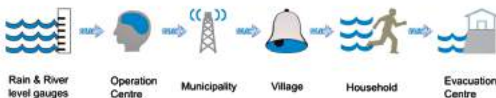
Figure 9.1 Schematic overview of the Binahaan LFEWS
