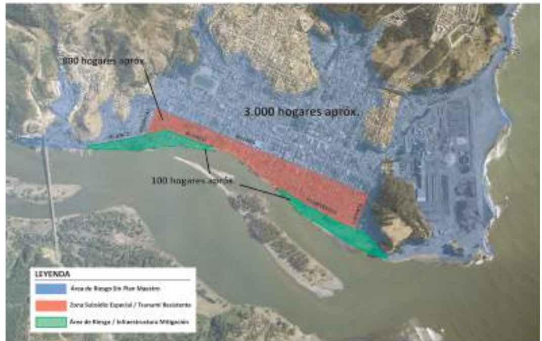
Figure 5.12: Constitución zoning plan, marking the flooding area for special subsidies for tsunami resilient designs
